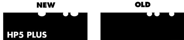
The new notch code, being phased in (September 1995) includes an ILFORD identifier. This identifier is an elliptical notch in the number one and number five positions. Either set of notches indicated above identifies ILFORD HP5 Plus sheet film.
