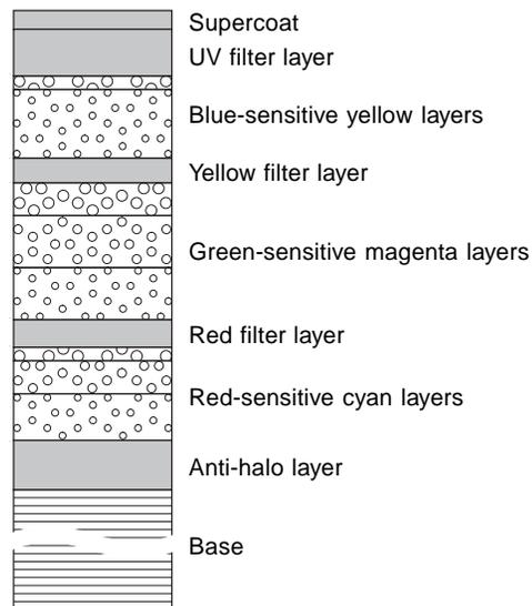
Total layer thickness (without base): 16 µm
